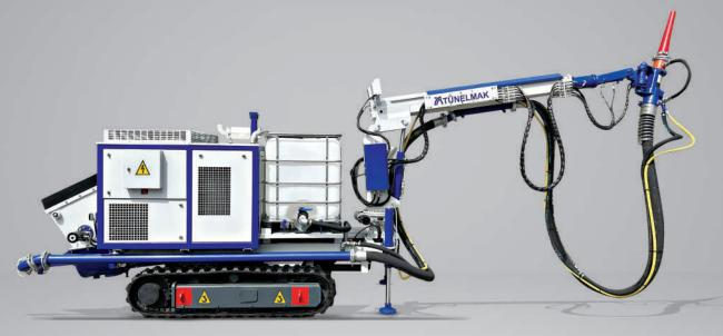
Adroit 016 DT is a shotcrete pump on crawler chasis with diesel engine. The machine have a concrete pumping capacity of 16m3/h. It is fully equipped with cable remote control for driving, concrete pump control and boom movements.
