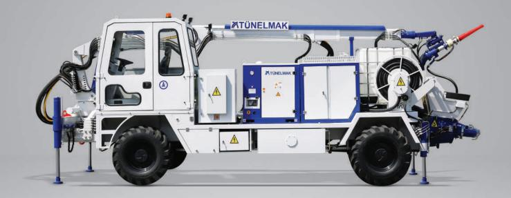
Adroit 450H/W series are designed as concrete pumping and shotcreting machines. The rigid chassis has 4 wheel drive and 4 wheel steering. Machines are fully equipped with lifting, tilting, telescopic boom system, rotation group, compact modular system, water & admixture pumps and tanks, energy cable reel, compressor on the platform. Standard pumping capacity is 30 m³/h, concrete pumping capacity is adjustable.
