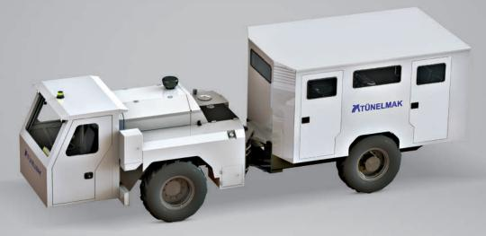
Adroit 618AW, which is designed for tunnels, mines and challenging field conditions, has made transport safer and faster in underground sites. 4x4 personnel carriers manufactured by considering the rough terrain conditions, have powershift transmission drive system on articulated chassis. It's available with fully-closed panel or glass-cab options. Although the standard carrying capacity of the vehicle is 16 + 2, this number can be decreased or increased depending on the demand of the user.
