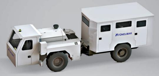
Adroit 618AW, which is designed for tunnels, mines and challenging field conditions, has made transport safer and faster in underground sites. 4x4 personnel carriers manufactured by considering the rough terrain conditions, have powershift transmission drive system on articulated chassis. It's available with fully-closed panel or glass-cab options. Although the standard carrying capacity of the vehicle is 16 + 2, this number can be decreased or increased depending on the demand of the user.
