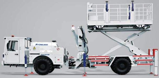
Adroit 641AW articulated scissor lift is designed as lifting and loading machine for tunnels and mines. The platform in the size of 3,8 m x 2,15 m has a bearing capacity of 2500 kg and can reach up to 4 meters height from ground surface.
