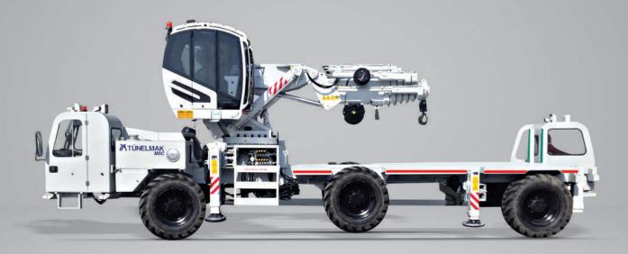
Tünelmak MSC is a vehicle which has a crane system on the chassis, designed to transport and unload all kinds of precast panels, railway panels and any material that may be needed in work areas such as tunnels and channels where width and height are restricted. The machinery has 4x6 hydrostatic drive system equipped with an operator's cabin from both rear and front. Six wheel steering system offers front wheel control and crab steering.
